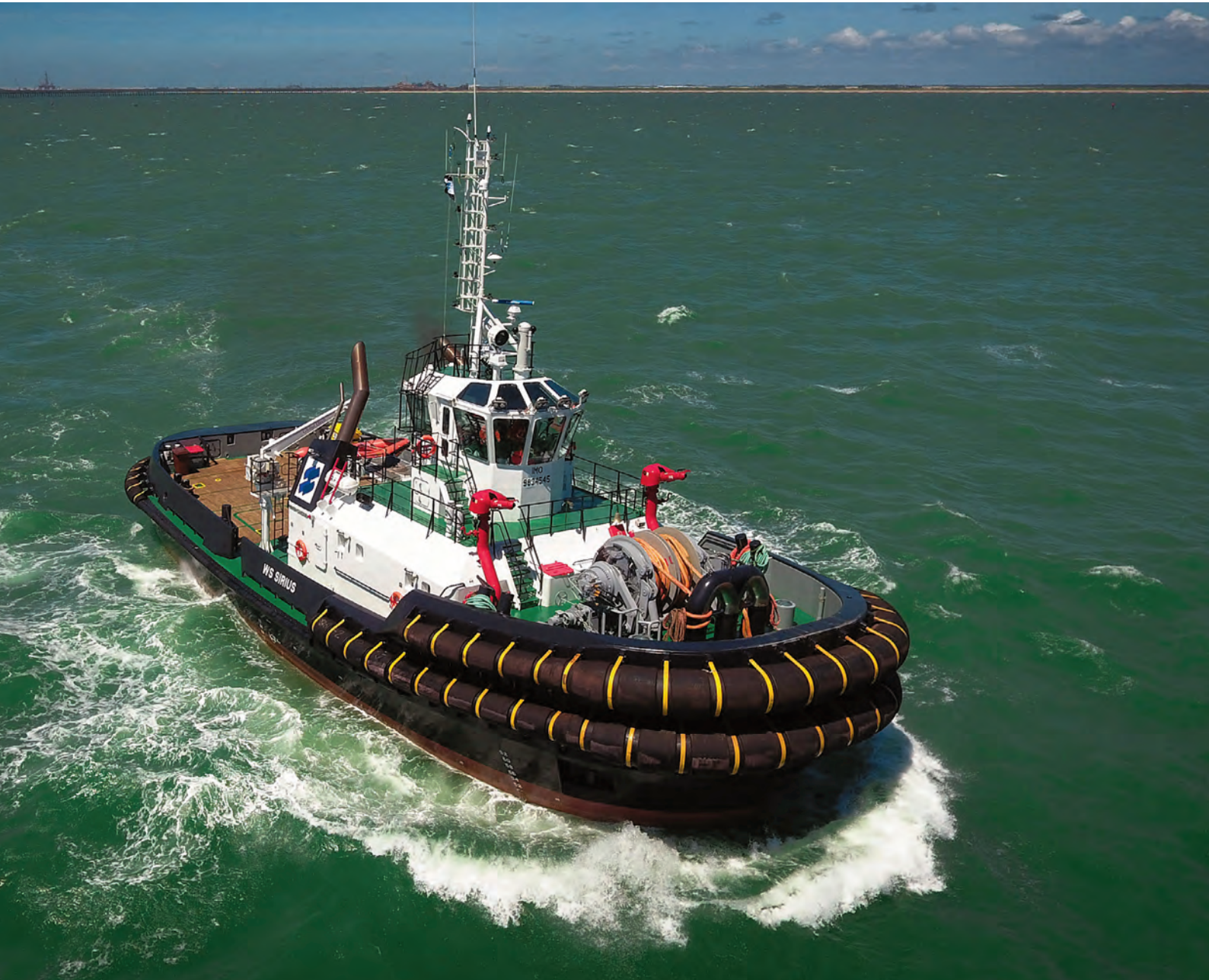
WS Sirius, a 90 ton bollard pull tugboat built at the Wilson Sons shipyards in Guarujá, São Paulo state, delivered in 2018. WS Sirius is the most powerful tugboat currently operating in Brazil.
